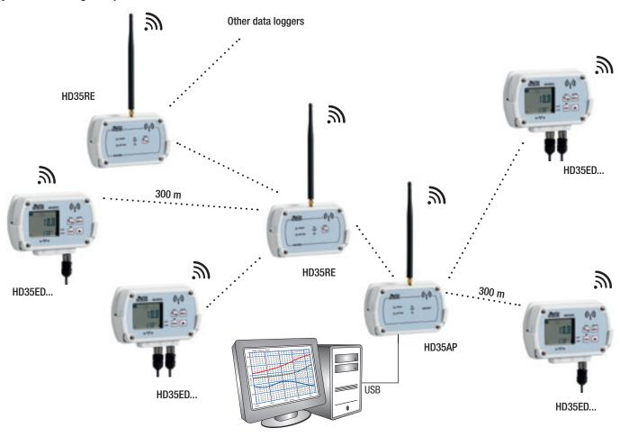
The system can consist of up to **255** devices (including the base unit and any repeaters). Each device is uniquely identified by its own address.
