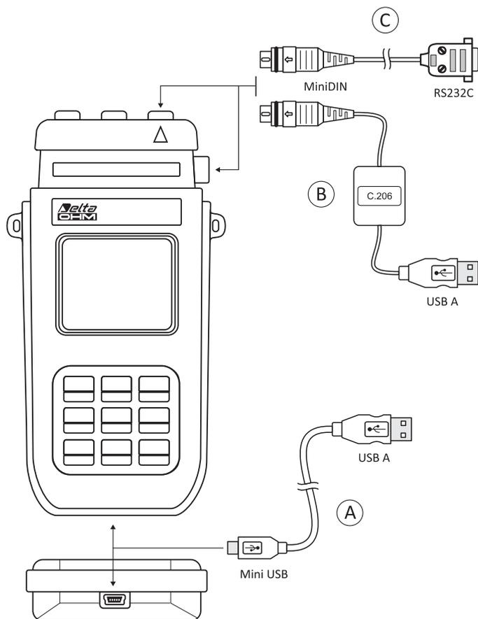
**A** To the portable data loggers of the series **HD21...2** a serial port mini USB type HID (Human Interface Device) has been inserted.
