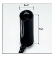
**LP 9021 LUM2:** Probe for measuring **LUMINANCE**, measuring range from 1 to 1999·10<sup>3</sup> cd/m<sup>2</sup>. Measuring angle 2°. CIE filter for correction of the response according to the human eye, CIE n°69-UNI11142.
