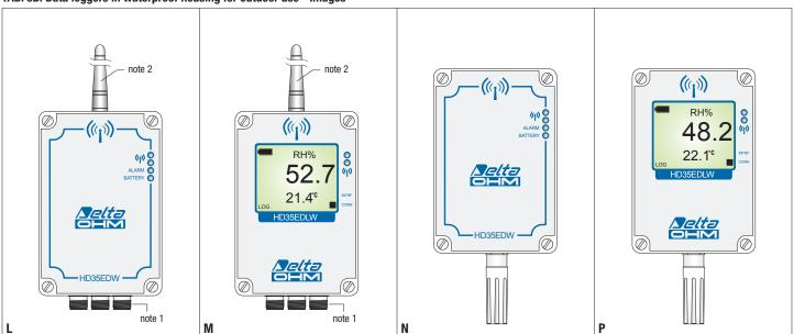
Note 1: the number of M12 connectors depends on the model and is indicated in table 6A.
