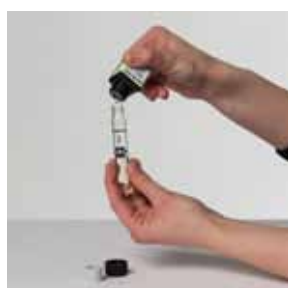
7) Add a defined number of drops of the colour reagent.
