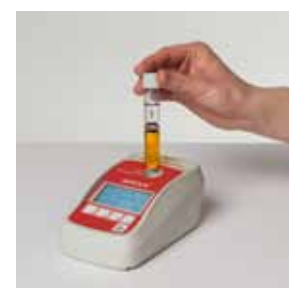
9) Insert the cuvette into the AMOLA® base unit. Read the measured value directly in kg/ha (mineral soils) or mg/l of substrate (for substrates), or ...
