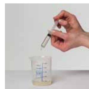
5) Measuring the filtrate with a graduated plastic syringe
