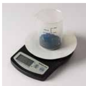
and: weighing the soil sample to determine the nutrient content in mg/kg
