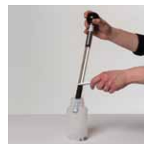
1c) Measuring the sample volume using the graduated sampling auger (e.g. for mineral soils)
