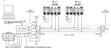
Line termination must be set at the two network ends. To polarize the line during non-transmission periods, resistors are connected between signal and power supply lines.
