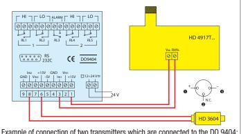
Example of connection of two transmitters which are connected to the DO 9404: a R.H.% transmitter which sends a current signal (4÷20 mA) a pressure transmitter which sends a current signal (4÷20 mA)
