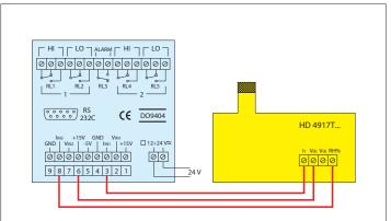
Example of connection of a passive transmitter which sends the D0 9404 two current signals ( $4 \div 20$  mA)
