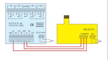
Example of connection of a self-powered transmitter which sends the D0 9404 two current signals (4 $\div$ 20 mA)
