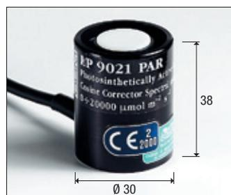
**LP 9021 PAR:** Quantum-radiometric probe for measuring the **PHOTONS FLOW** in the chlorophyll field PAR (photosynthetically Active Radiation 400nm...700nm), μmol·m<sup>-2</sup>·s<sup>-1</sup> measure, cosine correction diffuser.
