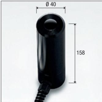
**LP 9021 LUM2:** Probe for measuring **LUMINANCE**, measuring range from 1 to  $1999 \cdot 10^3$  cd/m<sup>2</sup>. Measuring angle 2°. CIE filter for correction of the response according to the human eye, CIE n°69-UNI11142.
