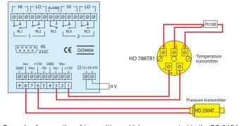
Example of connection of transmitters which are connected to the D0 9404: a temperature transmitter which sends a current signal (4÷20 mA) a pressure transmitter which sends a current signal (4÷20 mA)
