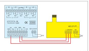
Example of connection of a self-powered transmitter which sends the DO 9404 two current signals  $(4 \div 20 \text{ mA})$
