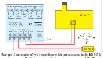
Example of connection of two transmitters which are connected to the D0 9404: a R.H.% transmitter which sends a current signal (4÷20 mA) a pressure transmitter which sends a current signal (4÷20 mA)
