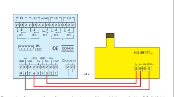
Example of connection of a passive transmitter which sends the DO 9404 two current signals (4 $\div$ 20 mA)
