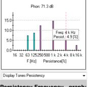
Persistency-Frequency graph: tonal components displayed as a function of their persistency **Equal-Loudness** CONTOURS: minimum spectrum of one or more components found, is compared to equalloudness con-Only the tours. band "touching" the higher isophonic curve is taken into account for calculation apply penalty.
