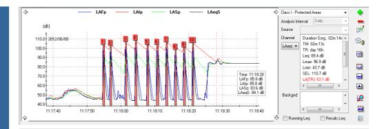
**IMPULSES DETECTION**: identification of individual impulses during Day and Night periods. Count associated to specific source or to the full measurement. Detected impulses are identified using markers and numbers on the time history and even in detailed tables. If the allowed number of impulses is excedeed, the LAeq,<sub>TR</sub> (Reference Period) will be added a 3dB penalty.
