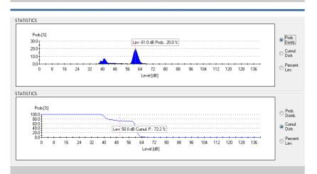
**STATISTICS:** from the measurement data it's possible to produce statistics as cumulative distribution, probability distribution and percentile levels. Statistical levels calculations are available as numerical and graphic format. Statistics can be processed also by individual sources.
