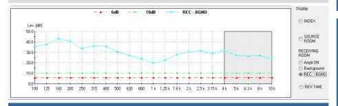
In order to verify that background noise doesn't influence the receiving room spectrum, it's possible a direct graphical comparison between background and received noise spectra. Obtained curve ( $L_{\text{Rec}}$  —  $L_{\text{Bgnd}}$ ) is compared to 10dB and 6dB thresholds as suggested in ISO technical standards.
